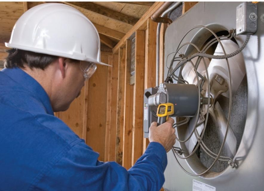
Check motor temperatures quickly, without contact.
