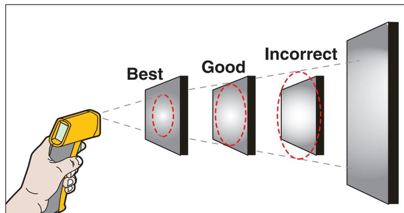
For the best readings, the measured target should be at least twice as large as the spot.
