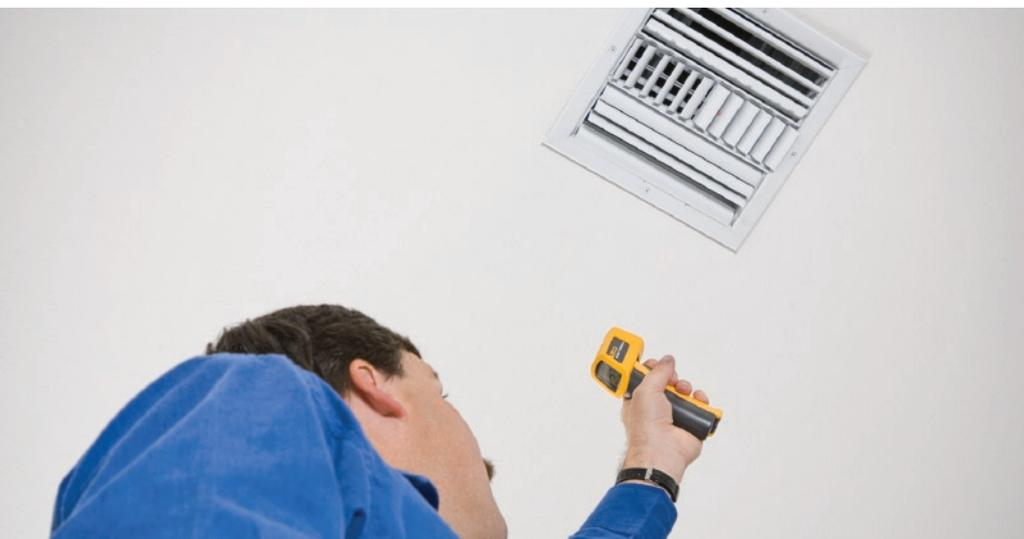
Use non-contact temperature measurements for inaccessible targets.
