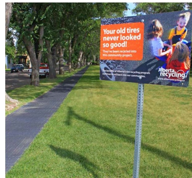
Sidewalk on north boundary of Heald Park. The concrete was replaced with recycled rubber blocks.
