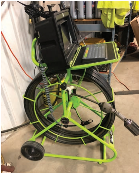
Sewer service line CCTV inspection camera
