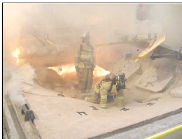
Figure 4: Floor Joist Collapse (National Research Council of Canada)
